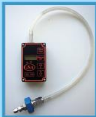
Purpose-designed particle impactor. Source: Keller, Fraunhofer IPA
